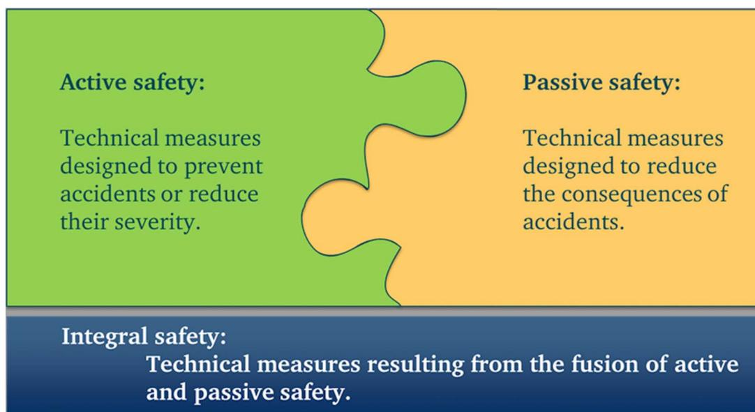
**Figure 2: Phases of the vehicular safety system ([i.70])**
