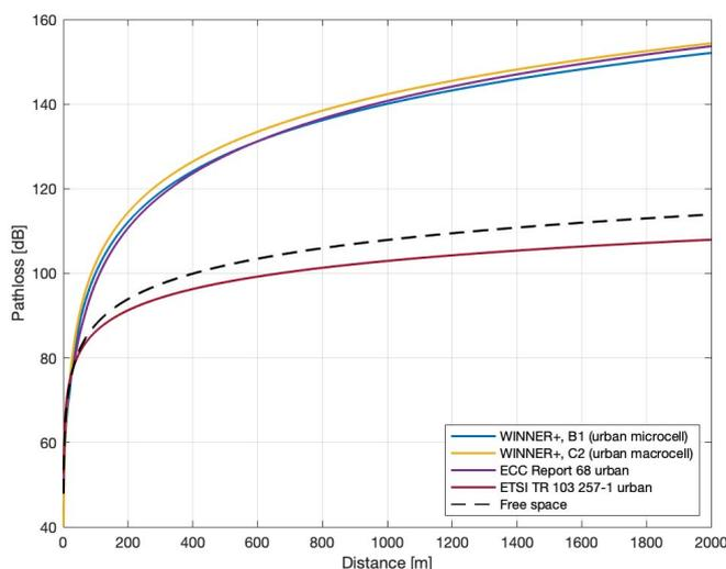
**Figure D.5-1: Path-loss vs. transmitter-receiver distance for a number of models designed for the urban scenario**
