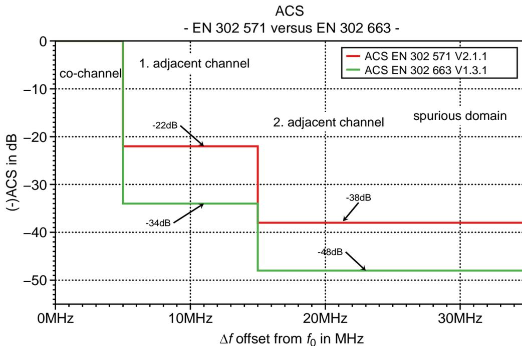
**Figure A.3-2: Adjacent channel selectivity ACS based on ETSI EN 302 571 [i.19] and ETSI EN 302 663 [i.22], QPSK with  $R=1/2$**
