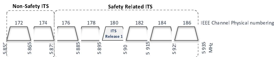
Figure 39: IEEE RLAN channel numbering [i.100]
