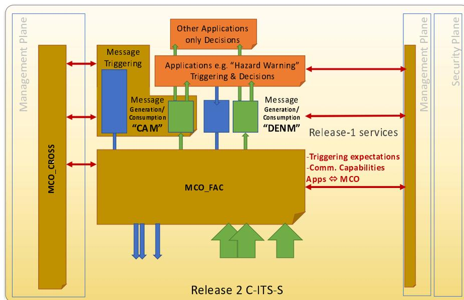
**Figure 9: Message triggering from out of Release 1 application or awareness service in a Release 2 system**
