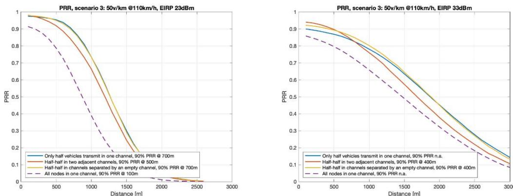
Figure E.4-1: PRR vs. distance in scenario 3 with packets of 550 bytes
