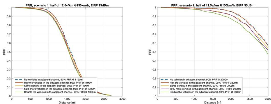
Figure 31 PRR vs. distance in scenario 1 with imbalanced traffic
