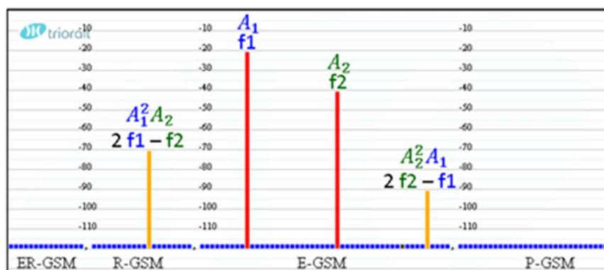
Figure 16: Generation of intermodulation products [i.106]
