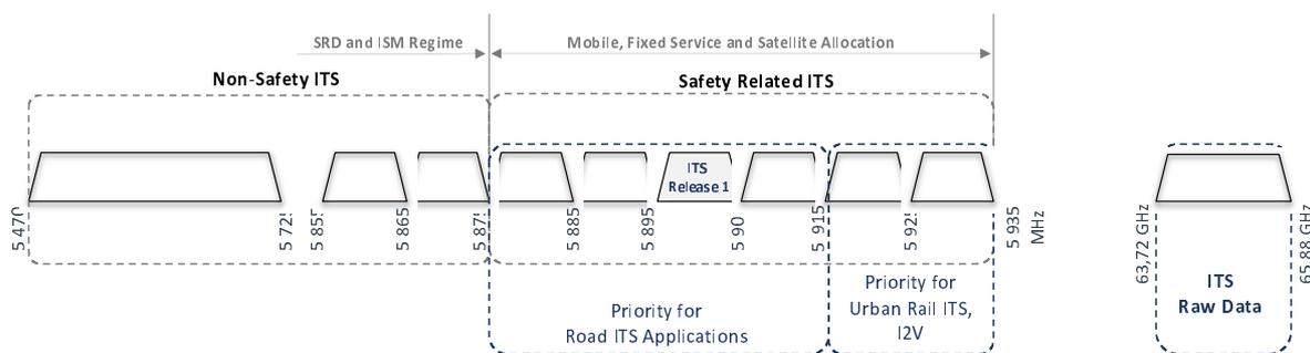
**Figure 4: Regulated ITS spectrum [i.73], [i.72] and [i.75]**
