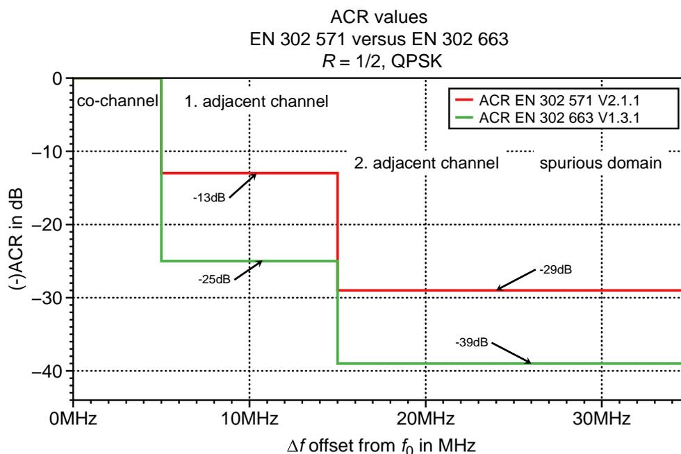
**Figure A.3-1: Adjacent channel rejection ETSI EN 302 571 [i.19] and ETSI EN 302 663 [i.22], QPSK with  $R = 1/2$**
