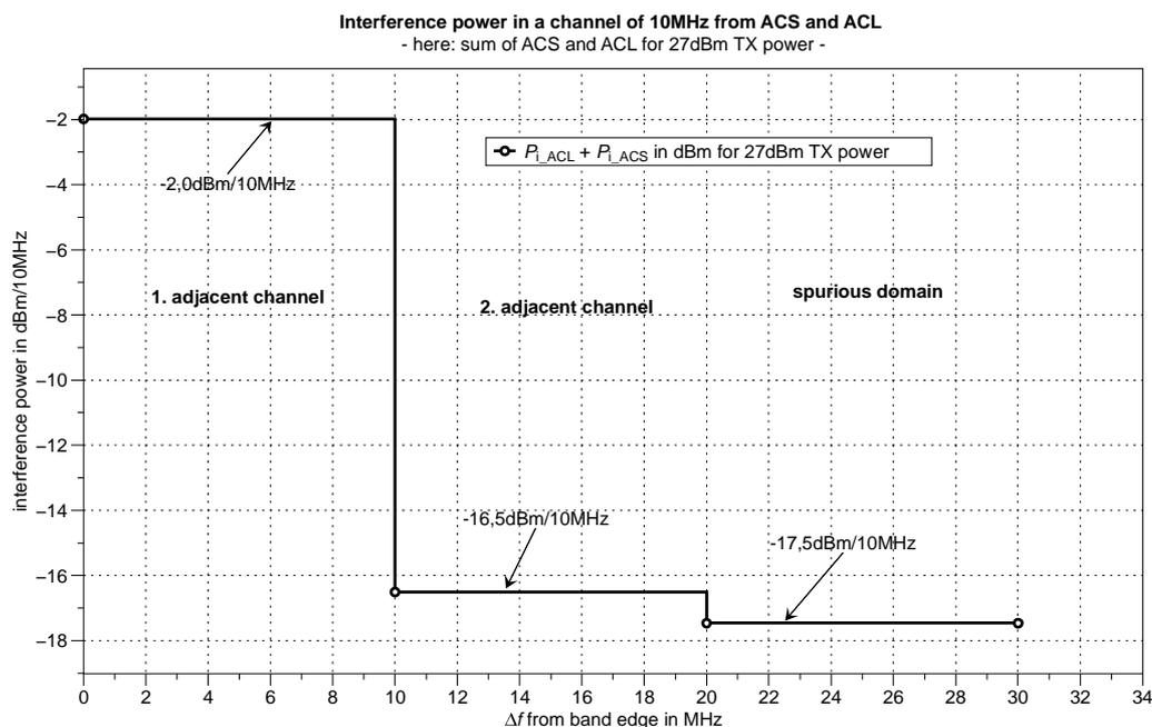
**Figure A.5-2: Example for ITS-G5: Effective interference power at the interfering TX  $P_{TX\_int\_eff}$  as combination of ACLR and ACS effect for 27 dBm TX power**
