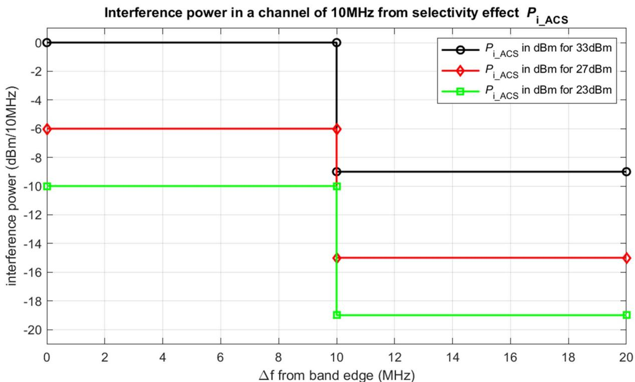
Figure B.3-2: Interference power in channel of 10 MHz from selectivity effect depending on received power level
