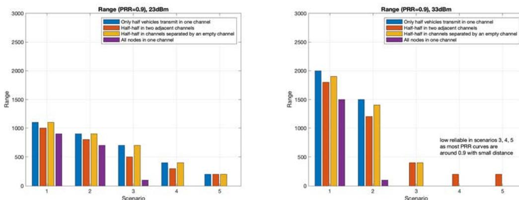
Figure E.4-3: Range (maximum distance with PRR = 0,9) with packets of 550 bytes
