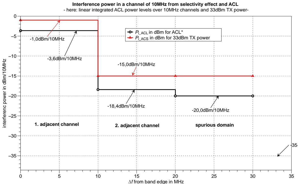
**Figure A.6-1: Example for ITS-G5: Comparison of ACS and ACL effects for 33 dBm TX power**
