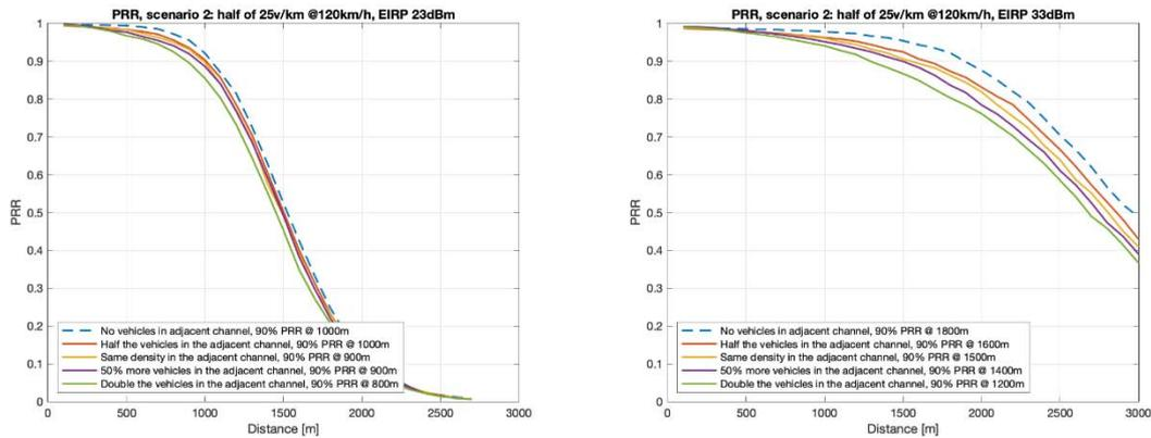
Figure 32: PRR vs. distance in scenario 2 with imbalanced traffic
