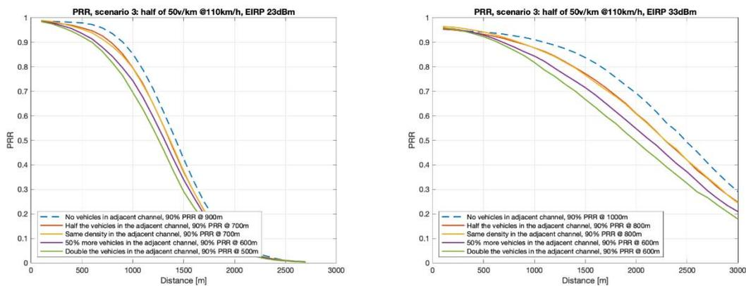
Figure 33: PRR vs. distance in scenario 3 with imbalanced traffic
