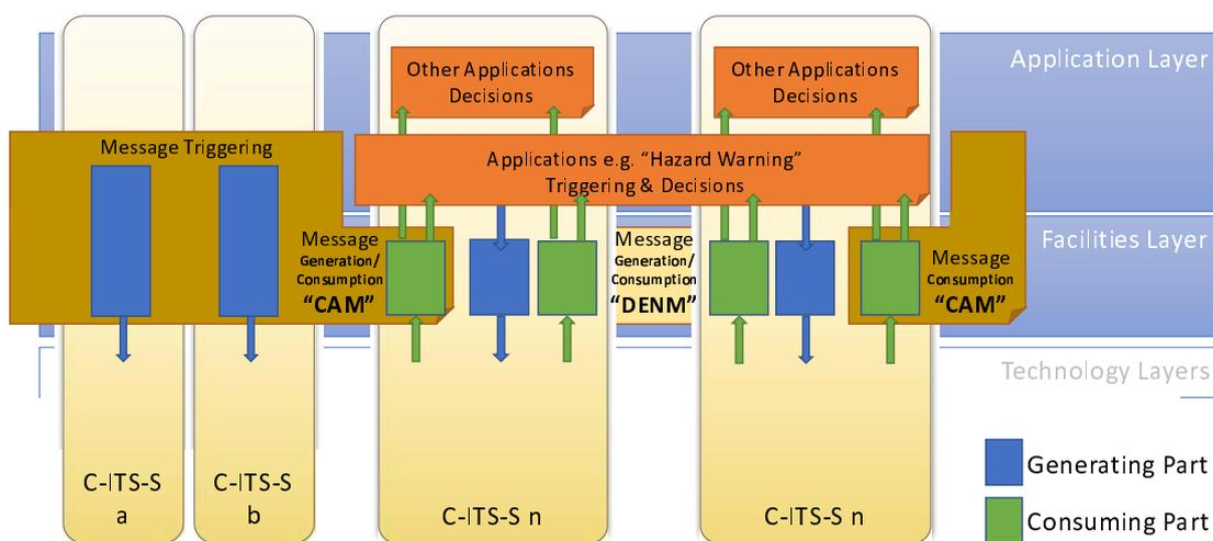
Figure 8: C-ITS application partitioning into generating and consuming parts in the various C-ITS-Ss
