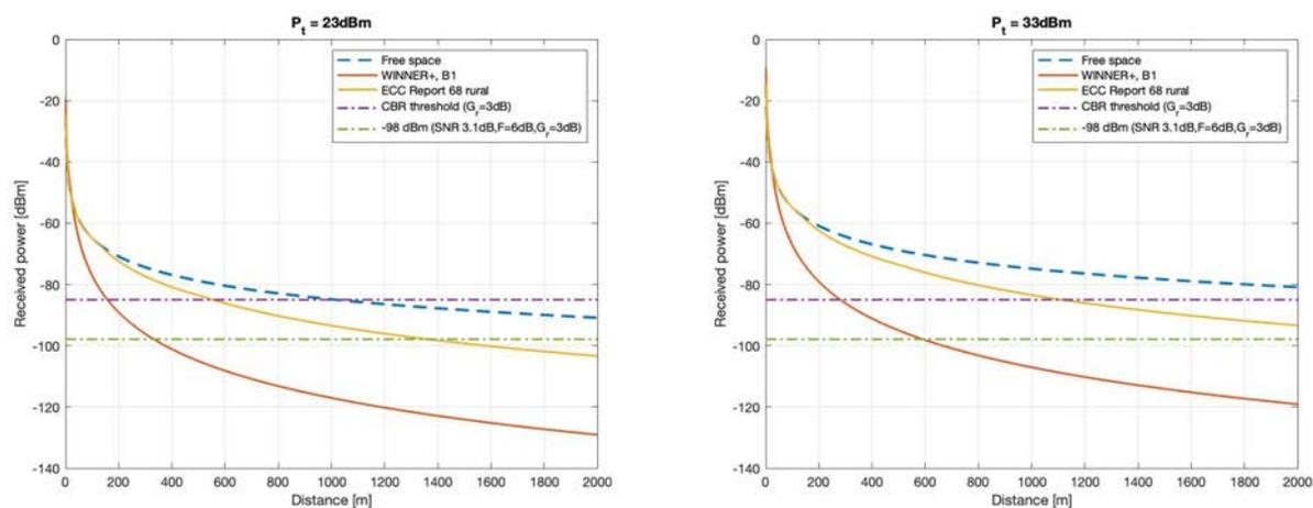
**Figure 21: Received power vs. the transmitted receiver distance assuming path loss only**
