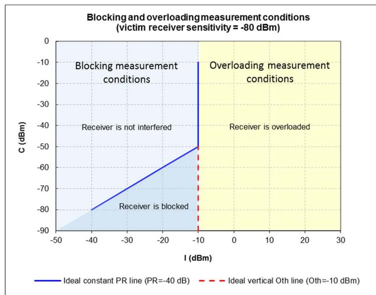
**Figure 15: Receiver blocking and overloading measurement ranges [i.106]**
