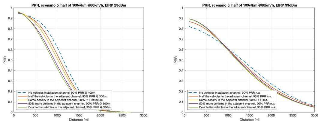
Figure 35: PRR vs. distance in scenario 5 with imbalanced traffic
