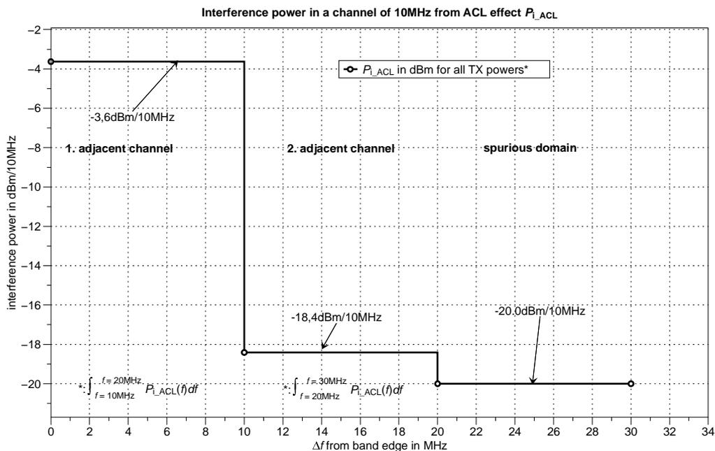
Figure A.4-2: ACL  $P_{1\_ACL}$  based on draft ETSI EN 302 571 [i.19]
