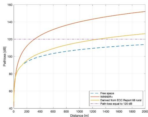
**Figure E.3-1: Path loss vs. distance with different models**
