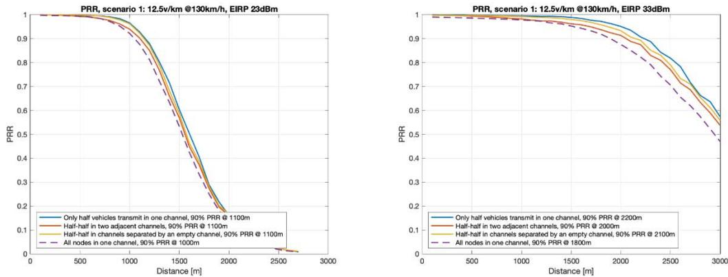
**Figure 23: PRR vs. distance in scenario 1 with balanced traffic**
