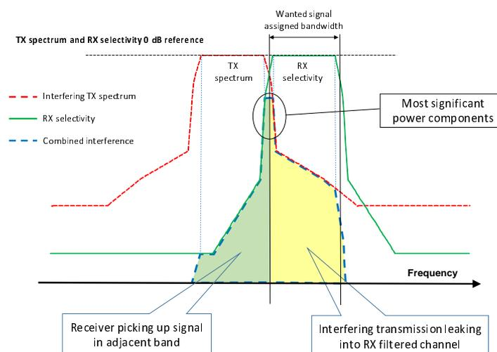
**Figure 14: Impact of an interfering transmitter and a victim receiver on the reception of wanted signals, see ECC Report 310 [i.106]**
