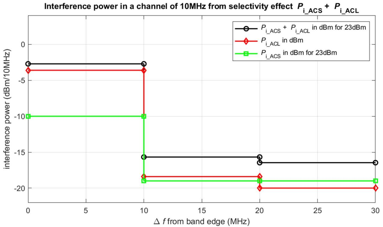
**Figure B.6-2: Aggregated interference power for 23 dBm**
