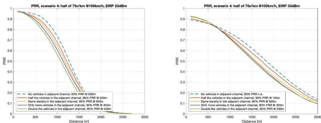
Figure 34: PRR vs. distance in scenario 4 with imbalanced traffic
