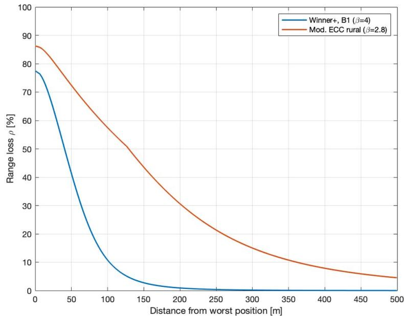
**Figure F.3-1: Range loss varying the distance of the vehicle from the position at minimum distance from the SRD**
