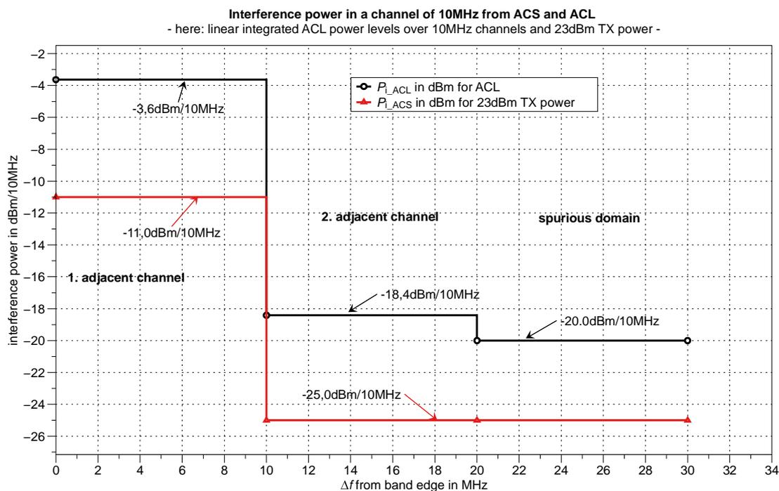
**Figure A.6-3: Example for ITS-G5: Comparison of ACS and ACL effects for 23 dBm TX power**
