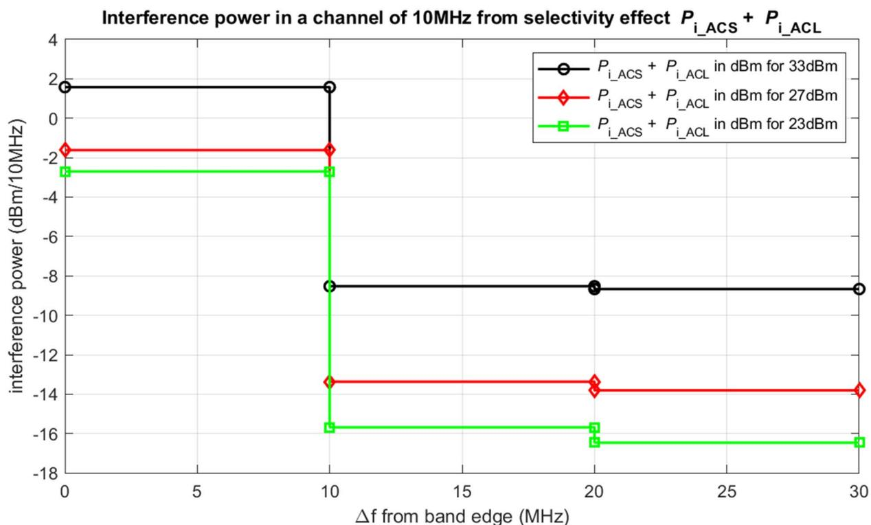
**Figure B.5-1: Example for LTE-V2X: Effective interference power at the interfering TX as combination of ACL and ACS effect**
