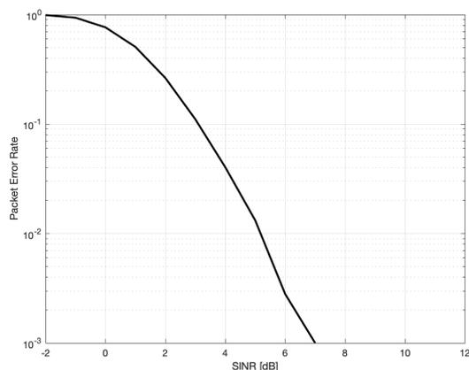
**Figure 20: Adopted curve of packet error rate vs. signal to noise ratio (MCS 2, 350 bytes)**
