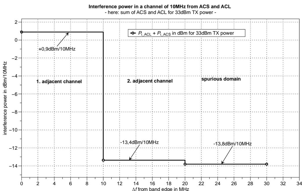
**Figure A.5-3: Example for ITS-G5: Effective interference power at the interfering TX  $P_{TX\_int\_eff}$  as combination of ACLR and ACS effect for 33 dBm TX power**
