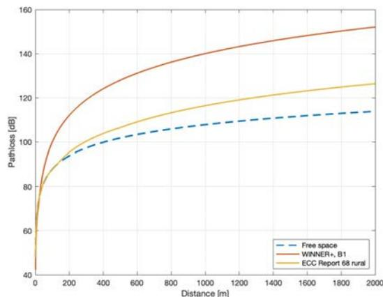
**Figure 19: Path loss vs. distance with ECC Report 68 [i.105] rural model and references**
