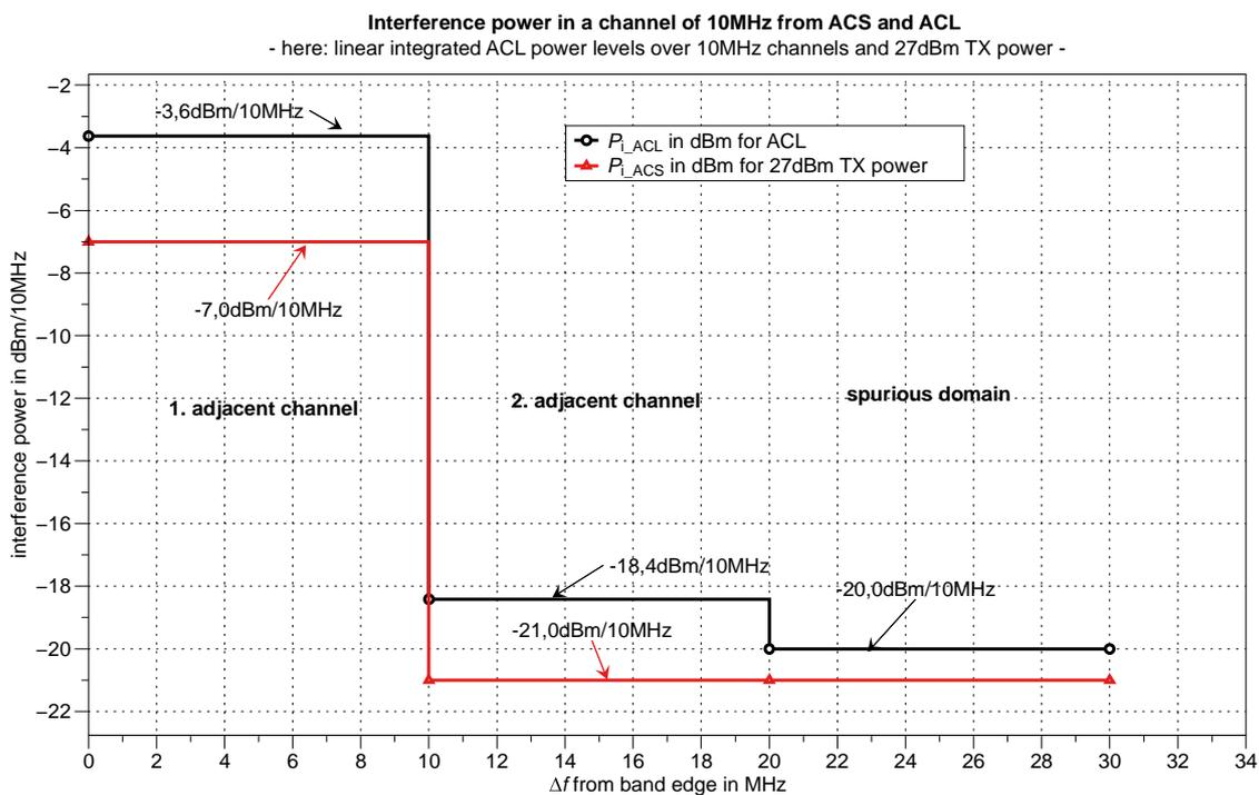
**Figure A.6-2: Example for ITS-G5: Comparison of ACS and ACL effects for 27 dBm TX power**
