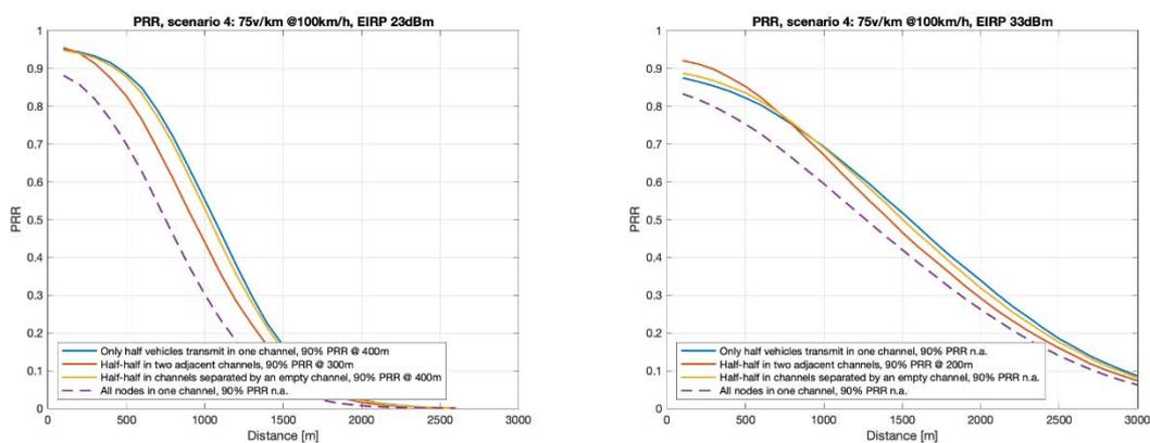
Figure E.4-2: PRR vs. distance in scenario 4 with packets of 550 bytes
