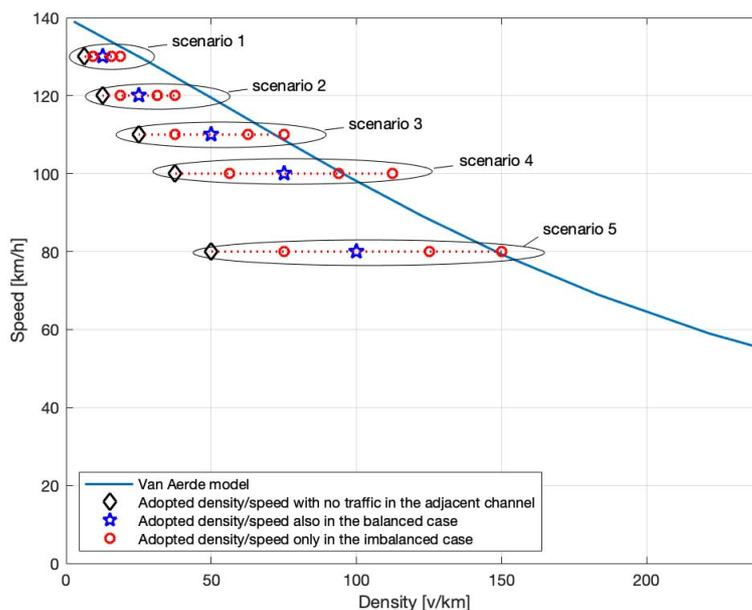
**Figure 30: Speed vs. Density of the scenarios investigated in the imbalanced traffic case**
