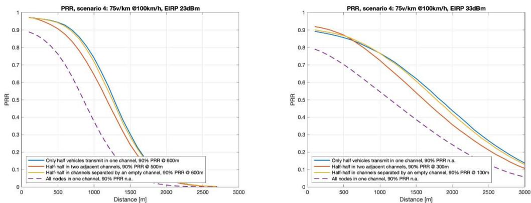
Figure 26: PRR vs. distance in scenario 4 with balanced traffic
