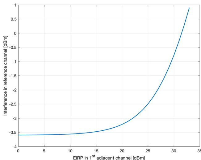
**Figure 38: ITS-G5; Interference power by a signal in an adjacent channel to a reference channel, varying the transmission EIRP, assuming the receiver is co-located with the transmitter**
