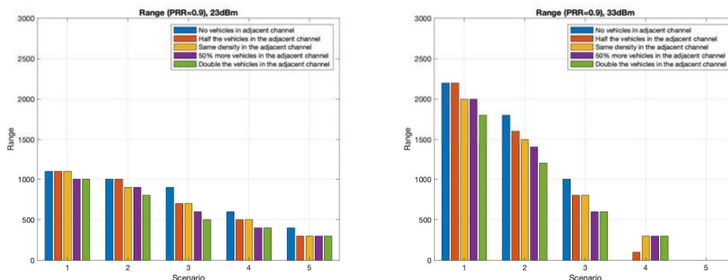
Figure 36: Range (maximum distance with  $PRR = 0,9$ ) with imbalanced traffic
