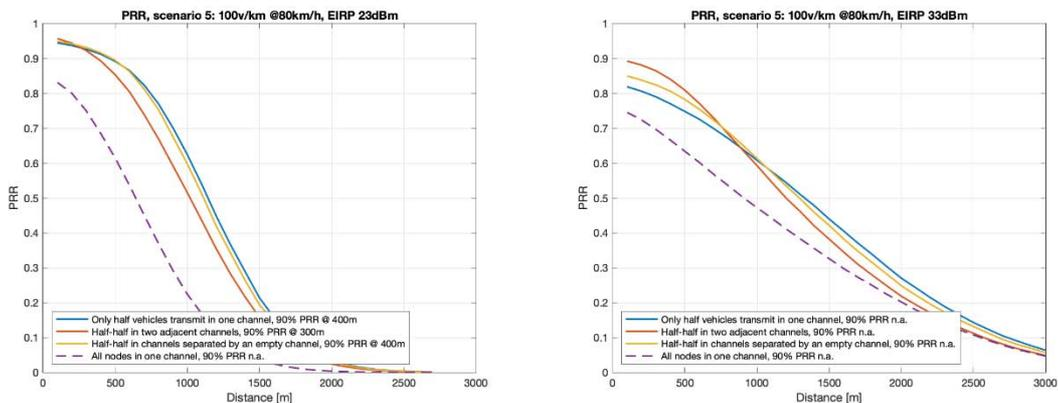
Figure 27: PRR vs. distance in scenario 5 with balanced traffic
