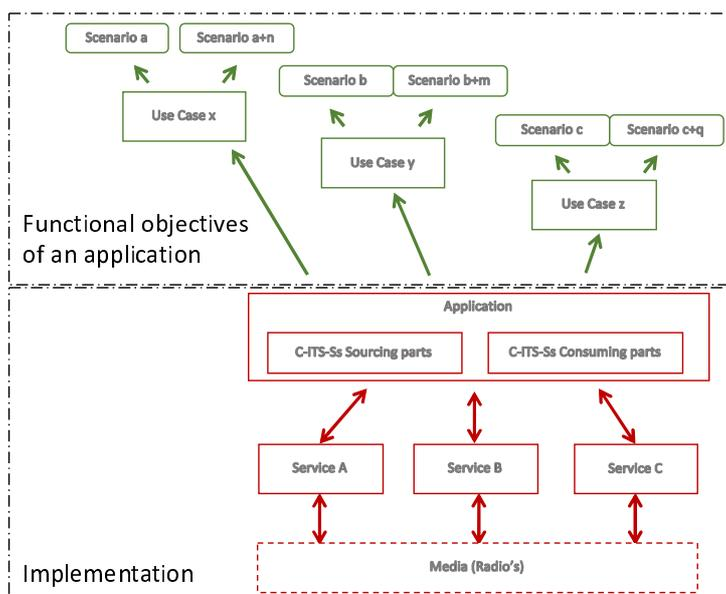
Figure 7: C-ITS application realizing use cases
