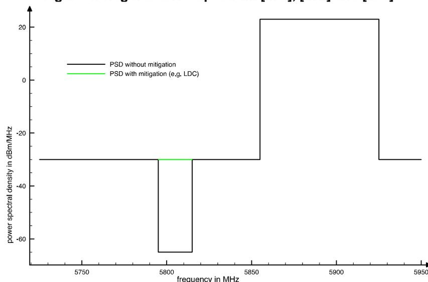
**Figure 5: Regulatory spectrum mask in ECC Decision (08)01 [i.72] and ECC REC(08)01 [i.73] in the year 2020 in dBm/MHz E.I.R.P.**
