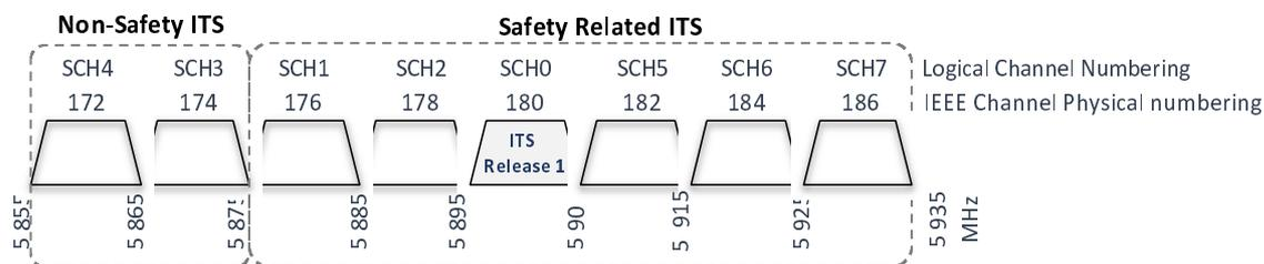
**Figure 43: Functional and physical channel numbering of the C-ITS bands**
