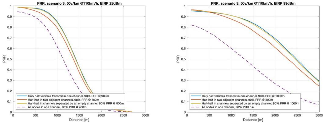
Figure 25: PRR vs. distance in scenario 3 with balanced traffic
