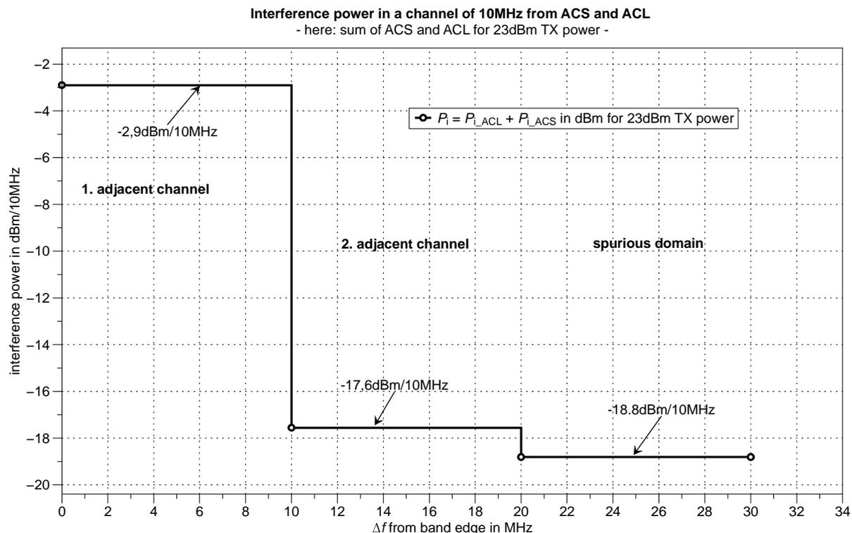
Figure A.5-1: Example for ITS-G5: Effective interference power at the interfering TX  $P_{TX\_int\_eff}$  as combination of ACLR and ACS effect for 23 dBm TX power
