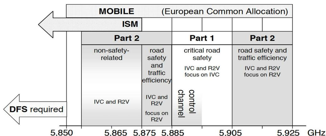
Figure 1: ETSI TR 102 492-2 [i.3] proposed spectrum allocation
