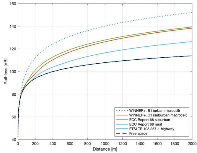
**Figure D.5-2: Path-loss vs. transmitter-receiver distance for a number of models designed for the highway scenario**
