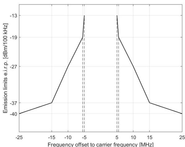
**Figure A.4-1: Transmitter spectrum mask draft ETSI EN 302 571 [i.19]**
